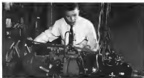
Automatic analysis test. General Electric tested the complete F-101A electric system prior to final airplane installation.
